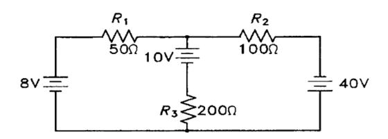
b. Determine the current drawn from the supply using start delta conversion. (5)
