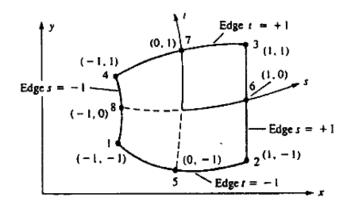
b. Derive the strain displacement B matrix for an isoparametric quadrilateral plate element shown on figure.
